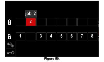
**Note:** The jobs which are disabled can not be using in "Save memory" function – shown in Figure 51 (job 2 is not available).
