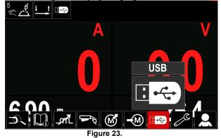
Press the Right Knob [36] to confirm the selection – the USB menu is shown on the display.
